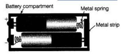
Connecting two cells together to make battery
